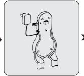
1- Fix four dowels on the wall2- Place four screws into their locations on the charging dock and mount on the dowels on the wall.
