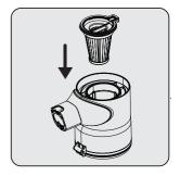
Attach pre-filter to the plastic filter back.
