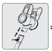
Push the tube in the direction of arrow towards the body by pushing on the tube release button.
