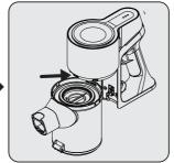
Fix the connector of dustbin to the holes on the body, then fix the dustbin until you hear the click sound.
