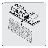
Attach mopping cloth to the bottom of water tank.
